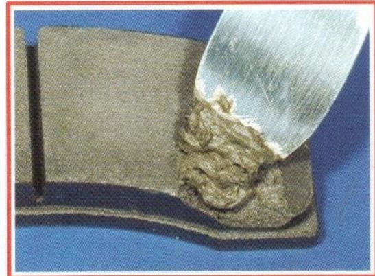
7032 Repairs a Wear Plate
